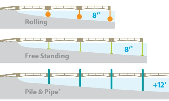
\*Maximum top of dock to lake bed with longest leg assembly. Calculate maximum water depth by subtracting distance required from top of dock to water line. Installations may vary, consult qualified ShoreStation dealer for proper applications.
